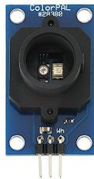
Figure 5: ColorPAL 28380 Sensor. Taken [2]
