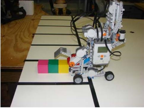
Fig. 7. Robot delivering cubes.
