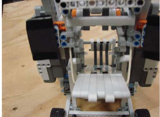
Fig. 1. Ramp inside the robot. The cube is dropped and carried on it.
