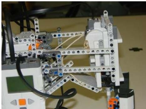
Fig. 3. Four-bar mechanisms and gears lifting claw.
