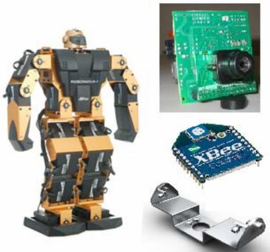
Fig. 4. Devices controlled by the new PCB and mechanical support for CMUCam2.
